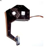
Place The Right Gripper assembly over the Lower Servo Plate assembly and secure together with the 5/8 inch 4/40 screws and nuts. The screws should pass through the Upper Servo Plate, Lower Servo Plate and the servo mounting holes.
