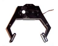
Place the Right Gripper over the square adjustable servo horn bracket and secure with the screw removed from the servo in step 1.
