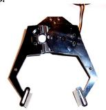
Trim to size the self adhesive foam pads and place on the ends of the gripper.
