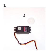
Remove the screw retaining the standard servo mounting wheel and replace with the square adjustable servo horn base.
